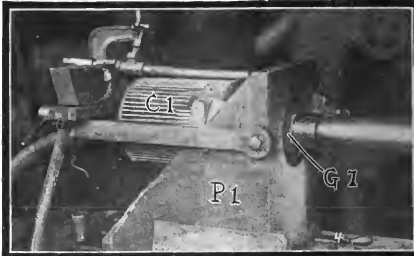
Fig. 2—In the Elmore Plant with a jiggling fixture G1 holding the manifold M1 on the platen P1 of a special drill so arranged as to accurately finish the four faces of the manifold M1 at one time.
